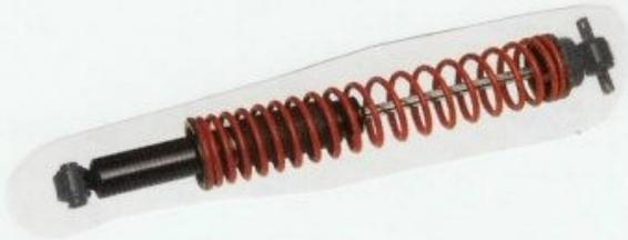
An elastic spring and a viscous damper combined as one unit is found in many common devices such as automobiles (termed struts) and storm door closers. In this strut the elasticity is clearly produced by the coil spring and the viscous damping by the fluid filled shock absorber. In tissue the demarcation is not so clear since the elastic and viscous properties result from a “blend” of various tissue constituents acting together.
